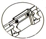
There is a U-Clip insert that fits between the clamp and the cable. This insert must be used to prevent damage to the cable. The lock actuators are adjusted and centered per the instructions, and the hexagon screws on the clamp are tightened.
